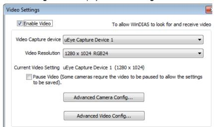
To save the settings you will need to tick the Pause Video tick box to enable the save settings options in Advanced Camera Config.
