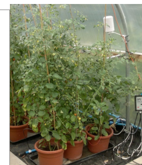
Fig. 2 – The experimental arrangement in the Delta-T polytunnel showing the close proximity of the air temperature and relative humidity sensor to the canopy together with air temperature and RH data over a 3 day period, used to calculate VPD by the GP2 Data Logger and Controller.
