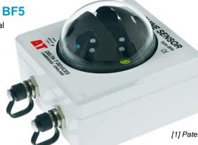
The BF5 uses this information to calculate whether the sun is shining and to measure the direct and diffuse components of solar radiation, avoiding the need for the shade ring adjustments required with conventional diffuse light sensors (levelling is the only adjustment required).
