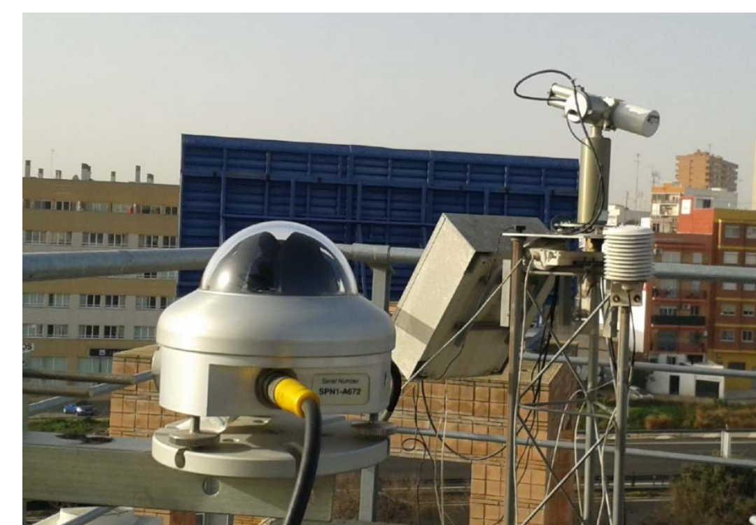
Figure 3. Close up on the SPN1 and sunphotometer at the site.
