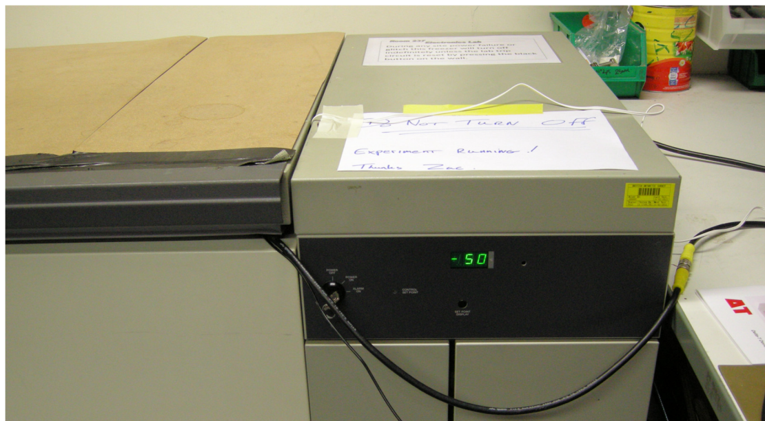
Figure 4 BAS Freezer at -50C showing the inline M12 connector in the SPN1 analogue cable. This connection was disconnected for 3 days to simulate 3 days without power at McMurdo
