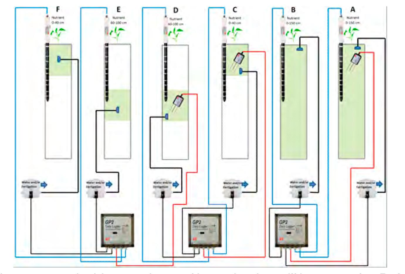
The next step in this experimental investigation will be to employ Delta-T's GP2 Advanced Logger and Controller with the WET Sensor and the PR2 Profile Probe to measure and log soil conductivity (nutrient level), soil moisture and temperature. Each GP2 is capable of providing precise closed-loop irrigation control at different soil depths when combined with the PR2, as well as fertigation control when combined with the WET Sensor.
