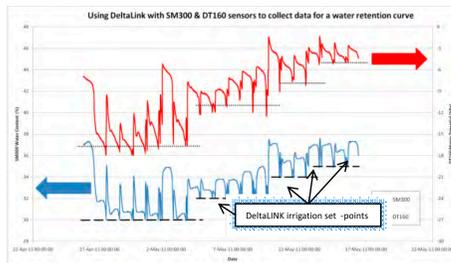
From the logger data above a water retention (drying) curve can be created by plotting the average of the matric potential sensor (DT160 dotted lines) against the soil moisture irrigation set point (SM300 broken lines) at the point of irrigation. This data can help identify a soil moisture range that avoids plant stress<sup>3</sup> and over-watering conditions. In the tomato plant study the irrigation set-point was set at 30% soil moisture.
