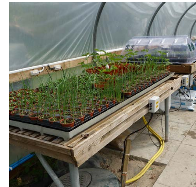
Fig. 4 – The flood tray, GP2 and propagators in the polytunnel at Delta-T Devices. In the experimental work shown here we have successfully used a dual propagator and flood trays system to grow
