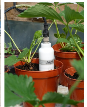
Fig. 5 – An SM300 Soil Moisture sensor providing VMC feedback for flood tray irrigation control.
