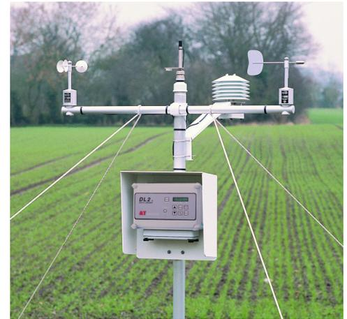
DL2e Loggers are well suited to meteorological applications. Delta-T can supply complete weather stations, including masts.
