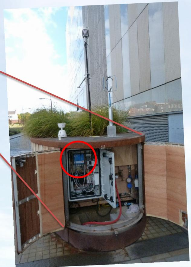
The GP2 logger circled opposite is installed at one end of a street side lysimeter. It can monitor a whole host of environmental parameters (from different types of sensors and from different manufacturers using analogue or SDI-12). One logger is in each of the 10 lysimeters with all data sent to a server and made openly accessible [here](#).
