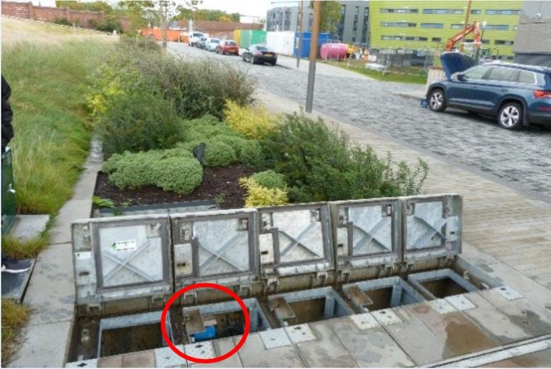
The image on the left shows a GP2 in a road side runoff monitoring installation.
